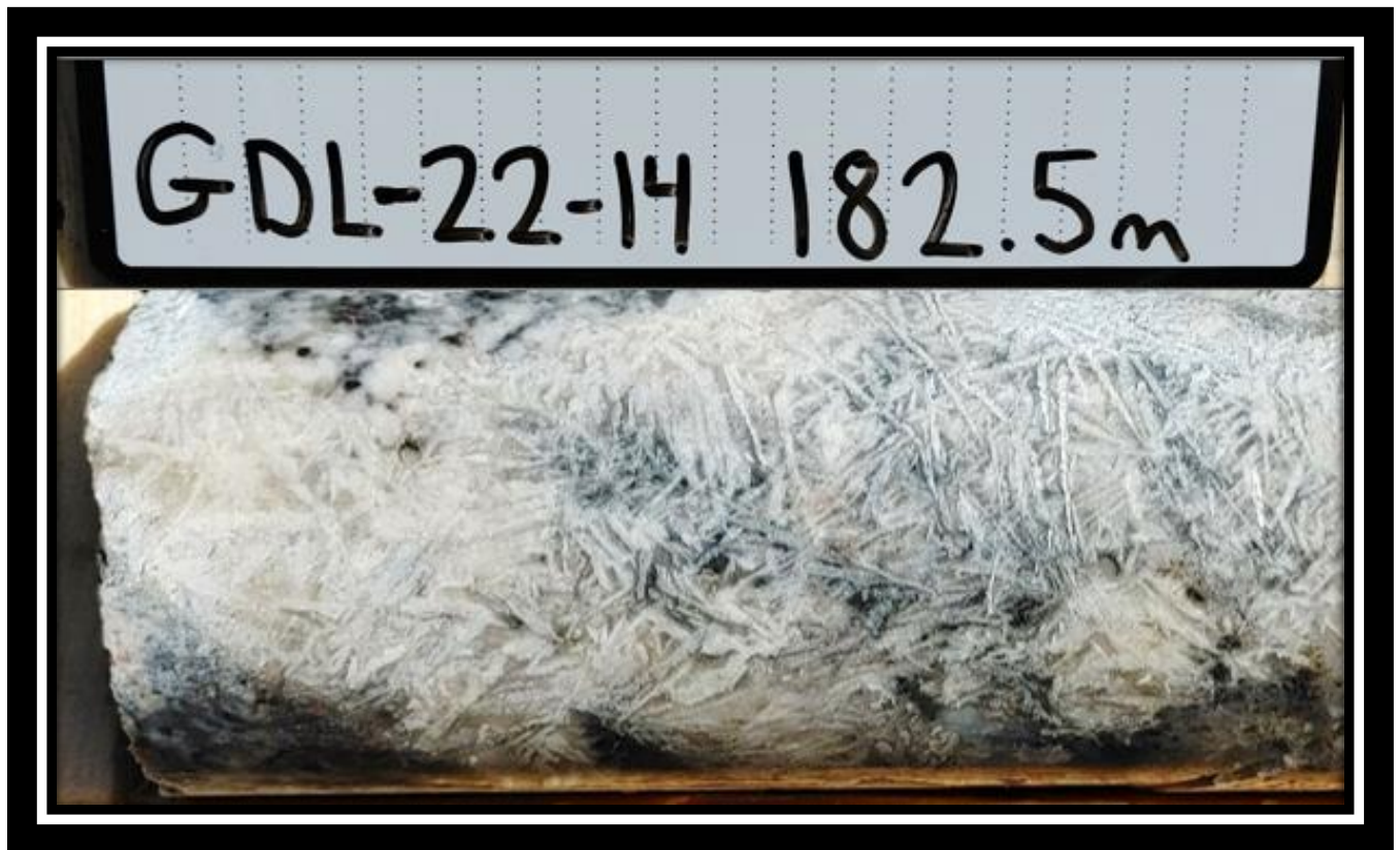
Above: Close up of elongate, white spodumene crystals in GLD22-14, drilled from the same setup as hole GDL22-13 reported on here. NQ core size.
