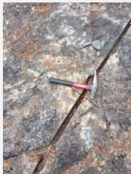
Right: Mineralized channel sample at South Rim area
