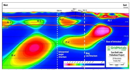
Above: cross section showing schematic of MT resistivity anomalies at Parisien Lake area.
