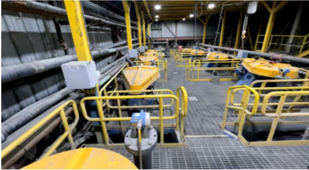
Figure 4: Flotation circuit at True North mill
