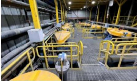
Above: Flotation circuit at True North mill
