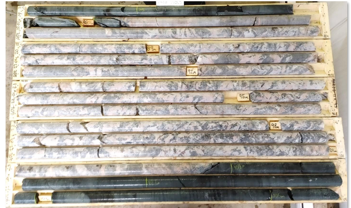
NW Dyke spodumene zone showing distinct coloration in comparison to surrounding country rock
