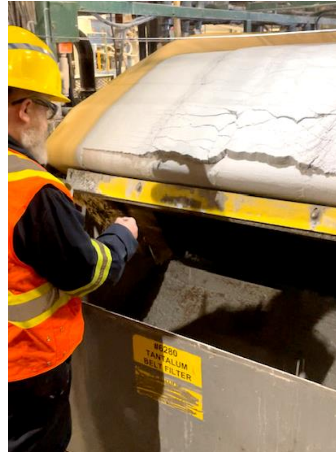
Above: Grid employee examining spodumene concentrate coming off filter press at Tanco Mine
