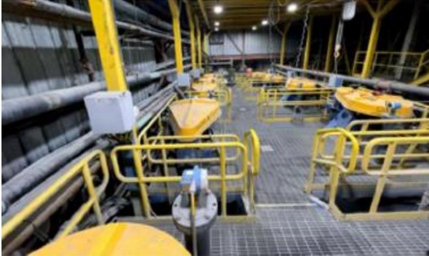
**Above:** Flotation circuit at True North mill
