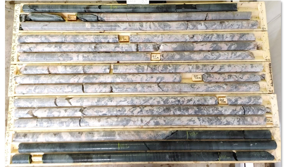
NW Dyke spodumene zone showing distinct coloration in comparison to surrounding country rock
